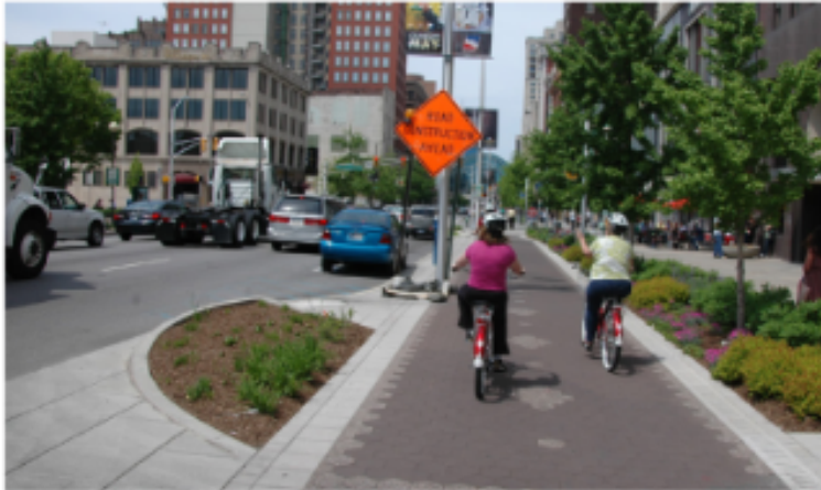
Raised separated bikeways are bicycle facilities that are vertically separated from motor vehicle traffic.
